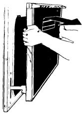
2. Grasp the door firmly at both sides and lift it up and away from the range.
